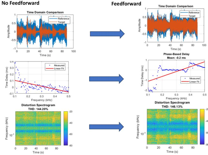
In our frequency sweep, using pure sin waves at different tones going through the arpeggio of a C Major scale, we identified a problematic frequency of C3, which is right at resonance. Our controller struggled with commanding this frequency, so we selected a song without this frequency. This can be thought as a notch filter eliminating that frequency, but in reality we just restrict to a song that doesn't have that frequency at all.
